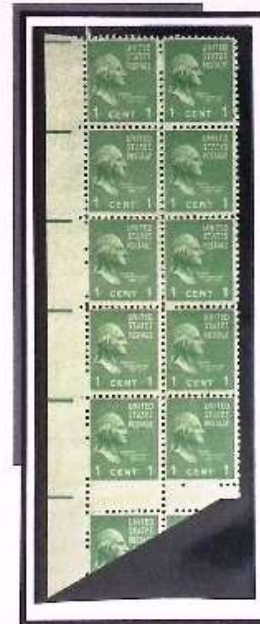
This interesting block of 10.5 was created as result of a strong paper fold that happened after the perforating process and before the final cutting process that reduced the production sheets to the service size of 100 units. The resulting vertical gutter snipe is a dramatic visual evidence of what can go wrong in the production process. (One must wonder if the rest of the sheet survived.)
